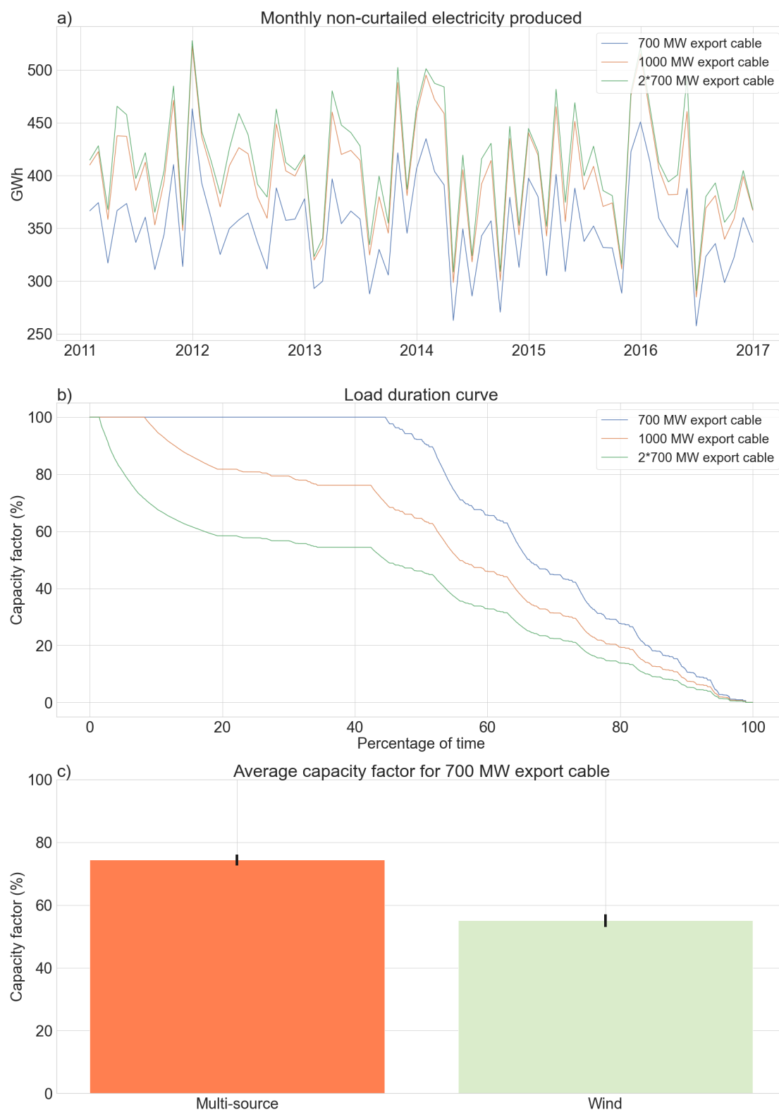
Figure 3: a) Monthly non-curtailed electricity produced based on three different export cables 700 MW (blue), 1000 MW (orange), and 2 x 700 MW (green). b) Load duration curve for three different export cables: 700 MW (blue), 1000 MW (orange), and 2 x 700 MW (green). c) Average capacity factor for multi-source (orange) and wind (green) for a 700 MW export cable. The black error bars show the standard deviation of the timeseries
